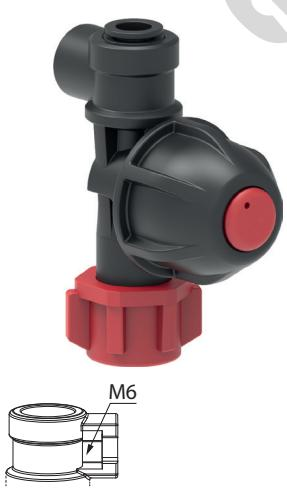
Portaugello con innesto rapido per tubo Ø 8 mm, antigoccia e testina filettata G 3/8" Nozzle holder with quick coupling for Ø 8 mm pipe, anti-drip and threaded cap G 3/8"
