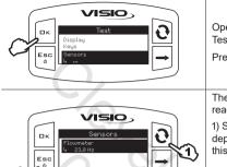
Open sensors test menu (Setup menu > Test > Sensors).
