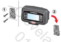
1) Set mounting rail in cabin and fasten it with the relevant screws (1), in a position where VISIO can be easily seen and at hands' reach, but away from any moving organs.
